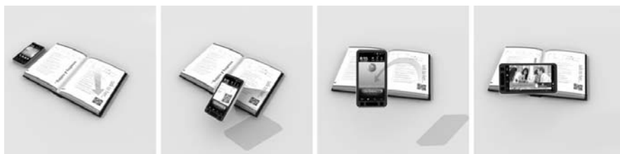
Figure 21-2. How QR codes work (steps 1-4)
