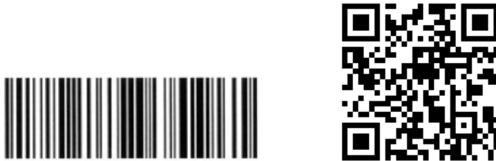
Figure 21-1. Samples of linear barcode (on the left) and QR code (on the right)
